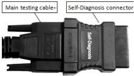
Main testing cable connects with self-test connector
